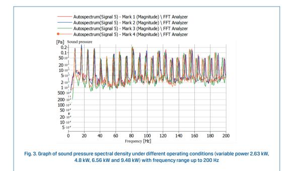
The analysis of the spectral density graphs (Figure 2, Figure 3) shows the dominant motor frequency of 12.5 Hz and the occurrence of iterative frequencies. The spectral density graphs showed that the decrease in the obtained acceleration values was primarily due to the lower energy transmitted through the engine pistons transformed from the chemical fuel energy.
