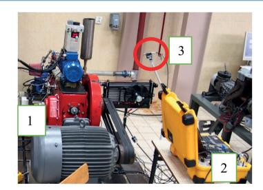
Fig. 1. Engine sound pressure measurement stand: 1 - Andoria Diesel engine S320 with CELMA Type 2Sf200 L6/4A electric starter-generator; 2 - Bruel & Kjaer sound record equipment; 3 - microphone
